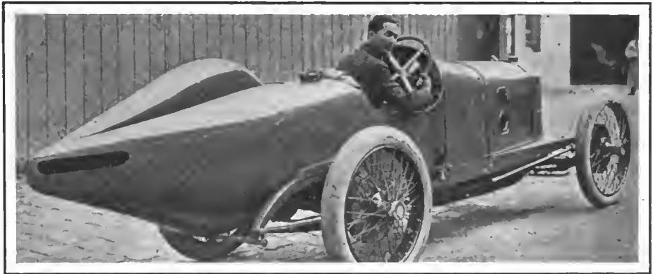
Goux on Peugeot Grand Prix racer. Note streamline tail to minimize wind resistance
